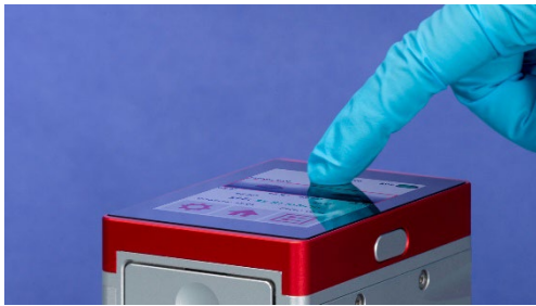
Picture 2: The PCA 200's integrated touchscreen makes it easy to control measurements and display the results.
